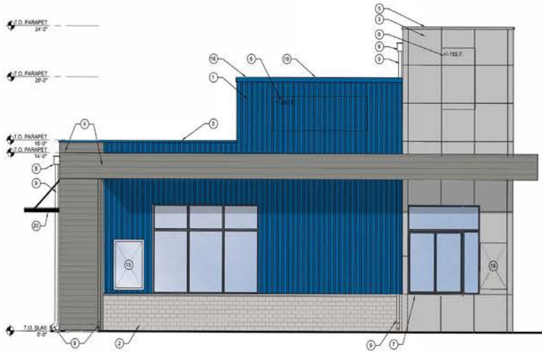
B EAST ELEVATION - DRIVE UP COFFEE SHOP SCALE: 1/4" = 1'-0"
