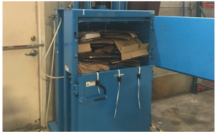
Recycling bailer in warehouse
