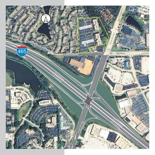
In the first quarter of 2012, during a 150 day period, the Allisonville/I-465 interchange will be reconstructed to be a single point urban interchange (SPUI). All I-465 ramps will be combined into one signalized interchange providing easy I-465 ingress and egress.
