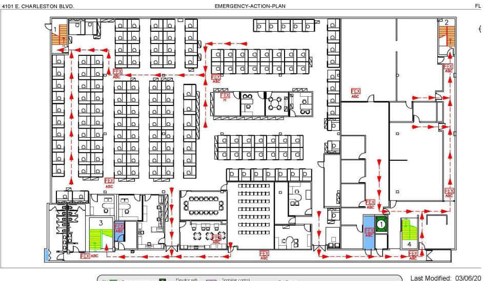
Elevator with identification Sprinkler control DN Tenant access stair ---- Exit Route w/area designation Fire Extinguisher; A=Class A B=Class B C=Class C Blind shaft with identification IBRA and designation Exit Stairwell Air supply D=Class D H=Halon Automated External Defibrillators Elevator Bank Stairwell Bank D Electrical closet Warden phone designation Fire Control Panels Standpipe Utility shaft Telephone closet Pull station Not to scale
