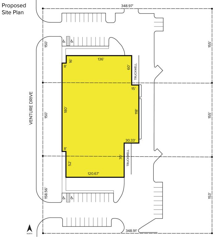
\* Suggested possible site plan allowing for required 100' rear setback.
