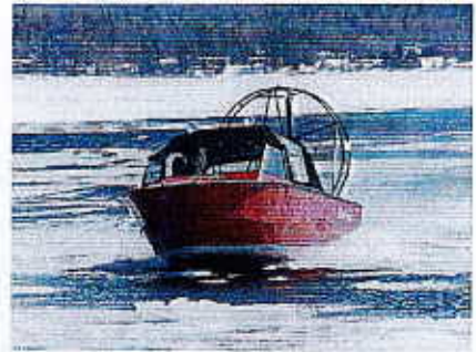
The Nattiq is the only airboat with positive flotation, a self bailing hull and U.S. and Canadian Coast Guard approved equipment.
