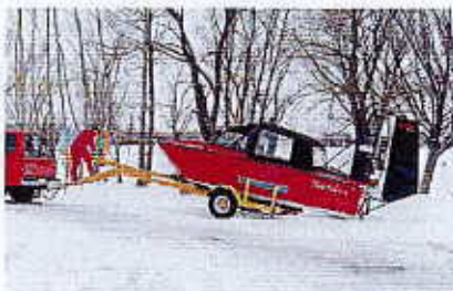
An optional tipping trailer can place the Airboat onto the snow without being unhitched from the towing vehicle.
