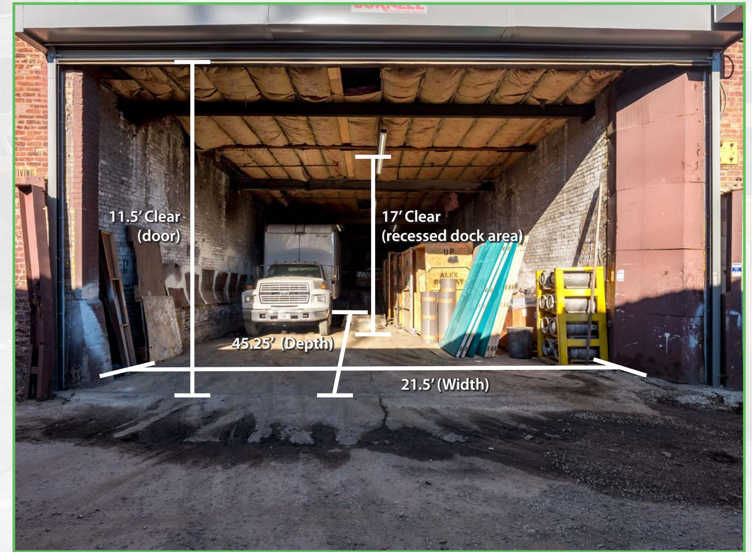
Recessed Loading Dock Dimensions
