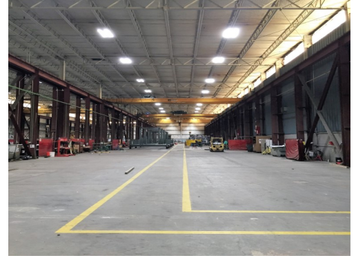
Bay 2 Two 25 ton cranes One 10 ton crane
