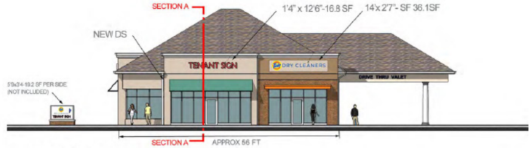
EAST ELEVATION 1 SF / LINEAR FOOT = 56 SF ALLOWED IN C2 DISTRICT SHOWN: 52.9 SF
