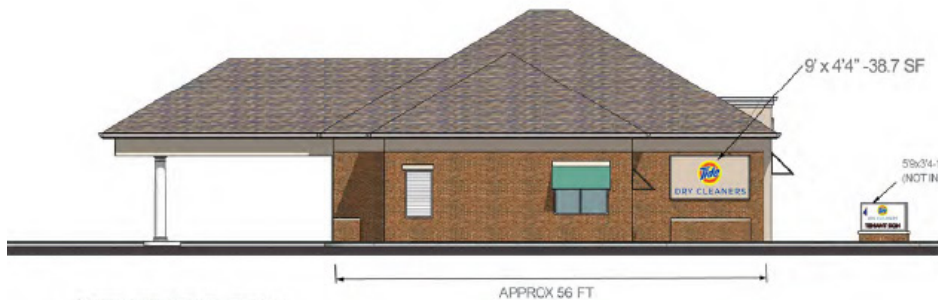
WEST ELEVATION 1 SF / LINEAR FOOT = 56 SF ALLOWED IN C2 DISTRICT SHOWN: 38.7 SF
