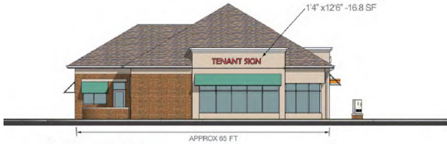
SOUTH ELEVATION 1 SF / LINEAR FOOT = 65 SF ALLOWED IN C2 DISTRICT SHOWN: 16.8 SF
