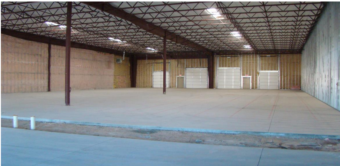
SPRINKLERED BLDG SHELL WITH 40'+/- COLUMN SPACING
