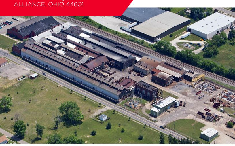
**210,338 SF** heavy industrial building utilized in the forging of components in all grades of stainless, alloy and carbon steel, titanium and other high-temperature materials. The forgings were principally made with closed impression dies and the facility has more than a dozen forging hammers, ranging from 1,500 to 25,000 lbs., as well as 6-, 3- and 4-inch upsetters. All forging equipment and supporting equipment are part of the sales price and transaction (full list of F, F & E available).
