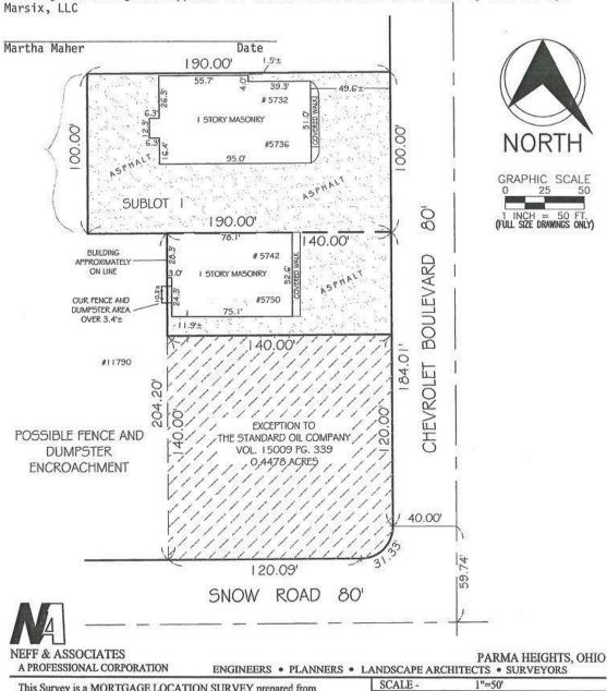
This Survey is a MORTGAGE LOCATION SURVEY prepared from actual field measurements in accordance with Chapter 4733-38 of the Administrative Code, AND IS NOT a boundary survey pursuant to Chapter 4733-37 of the Administrative Code.
